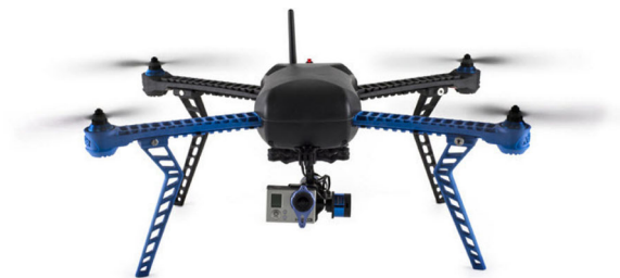
Fig. 1 The IRIS quadcopter with a GoPro camera mounted on a Gimbal stabilizer
