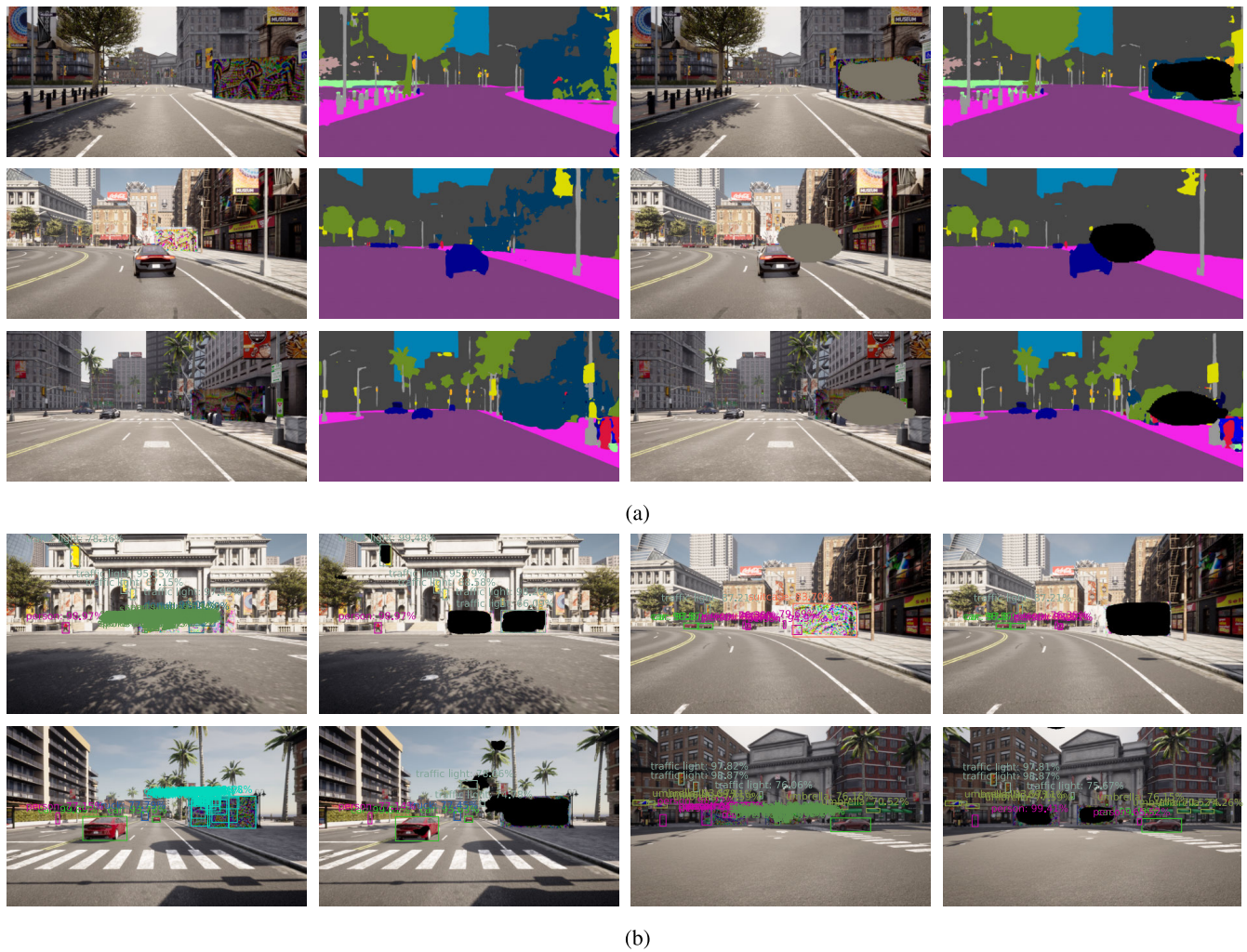
Fig. 8. Illustration of the effectiveness of adversarial billboards (column one and two) and of Z-Mask [24] (column three and four) for Semantic Segmentation (a) and Object Detection (b). Images are extracted from the generated datasets.
