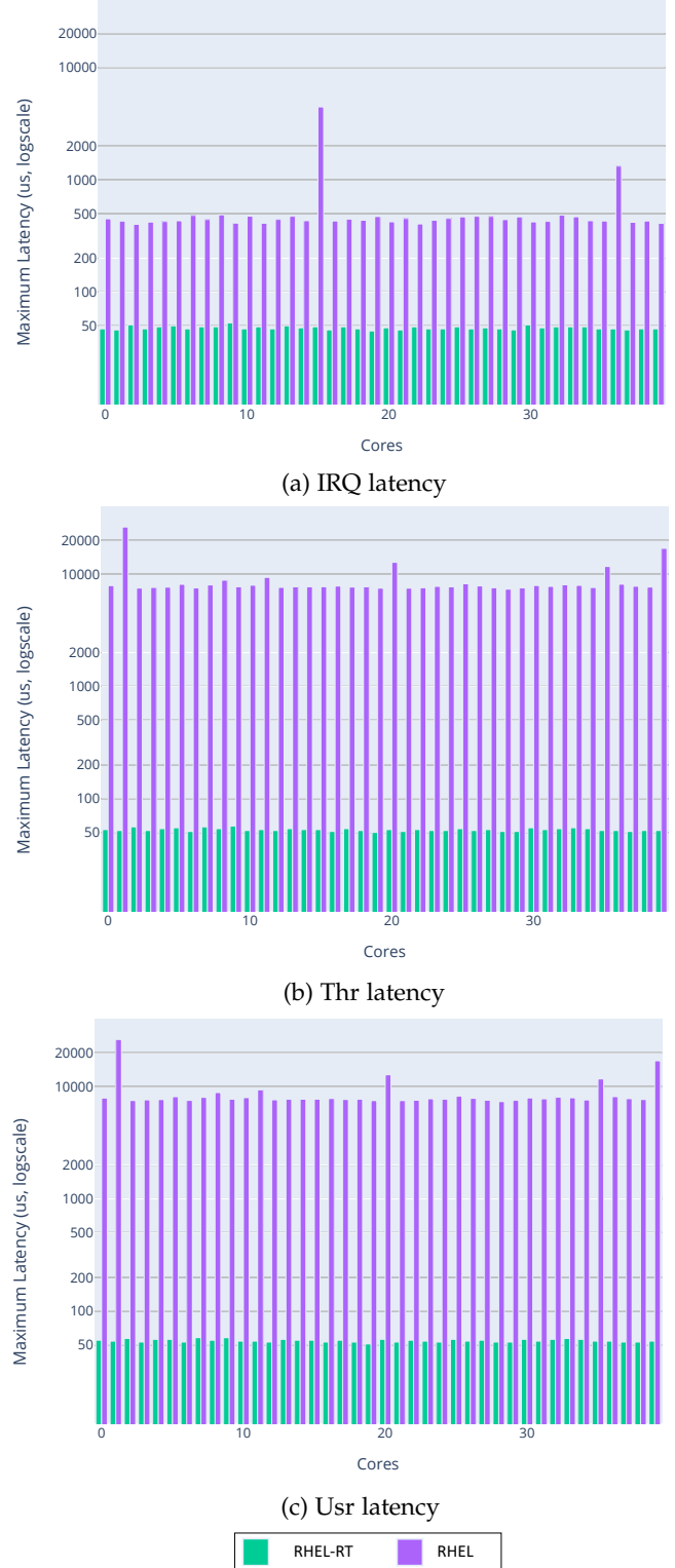
Fig. 15: Bar chart of the maximum latency values (logscale) obtained by running Timerlat for 6 hours in the workload configuration on 40 cores running RHEL (in violet) and RHEL-RT (in green).
